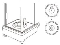
**bubble right above** clockwise rotate two leveling feet
