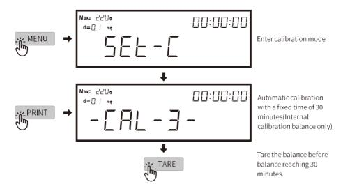
Remark: Balance should keep "0.0000", Tare the balance if balance not shown "0.0000" when reach 30 minutes.
