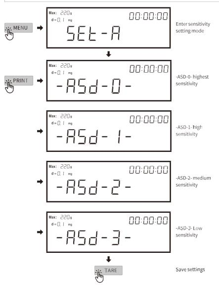
REMARK: factory setting sensitivity "-ASD-3-", suitable for most using environment. Higher sensitivity required better environment. Do not adjust the sensitivity without consulting the factory.
