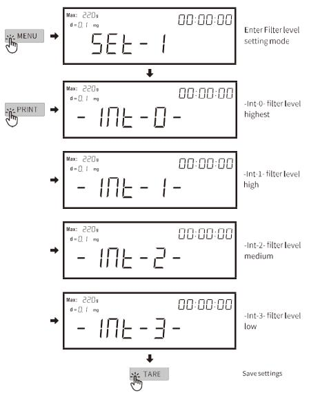
REMARK: filter level is the internal calculating time of balance, factory setting is "-Int-3-", do not change by yourself without professional instruction.
