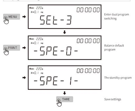
Remark: when switch to another program, please make a linear calibration again to unlock the balance.
